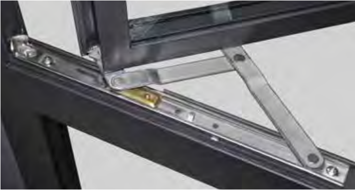
Concealed Friction Hinge (Stainless Steel) Available on Push-Out, Awning, and Hopper. Weight limit 120lbs.
